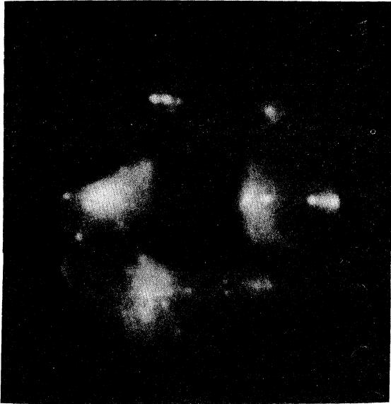
FIG. 7. LEED pattern from the silicon (111) 7 \times 7 surface with one monolayer of aluminum deposited at 600\text{--}700^\circ\text{C} . The primary electron energy is 45 eV.
