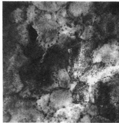
FIG. 1. Transmission electron micrographs of \text{LiAlSiO}_4 glass-ceramics with 2.8-mole% \text{TiO}_2 as a nucleating agent. (a) Micrograph of the 13% crystalline material with \sim 0.3\text{-}\mu\text{m} crystallites of \beta eucryptite; (b) micrograph of the 81% crystalline material with 1.2\text{-}\mu\text{m} crystallites of \beta eucryptite. The small dark areas located primarily in the grain boundaries of the \beta eucryptite crystallites [in part (b)] are \sim 50\text{-}100\text{-}\text{\AA} \text{TiO}_2 crystallites.
