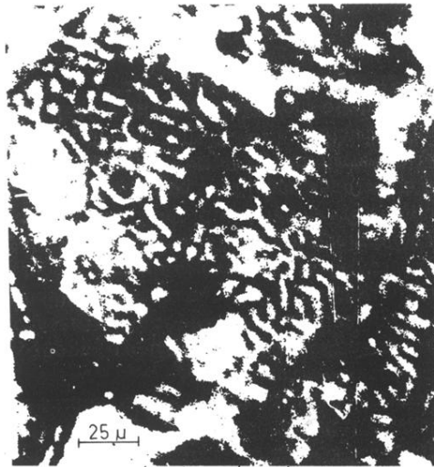
FIG. 3. Domains in a type- B crystal in an applied field of 280 Oe at T = 2 K.
