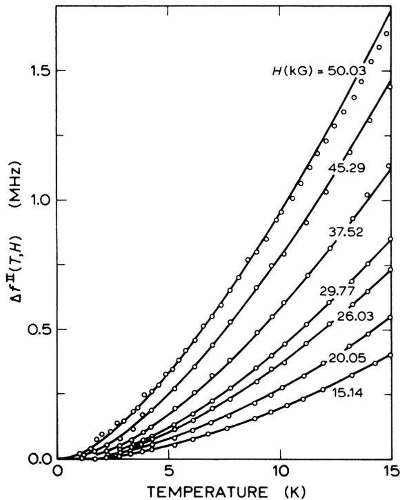
FIG. 6. Net magnetization, as reflected in the NMR frequency of the in-layer  $^{19}\text{F}^{\text{II}}$  nuclei corrected for the Zeeman shift  $\Delta f^{\text{II}}(T, H)$  vs temperature for various fields parallel to the  $c$  axis. Renormalized spin-wave theory (solid lines) has been adjusted to the data points below 30 kG and 15 K to determine the hyperfine coupling constant  $A_2$ .
