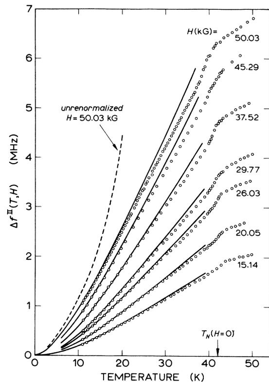
FIG. 7. Same as Fig. 6, but over a wider range of temperature. The part below 15 K is enlarged in Fig. 6. The solid lines are calculated from renormalized spin-wave theory, as described in text. The dramatic effect of renormalization is exemplified by the dashed curve representing unrenormalized theory at 50.03 kG with the effective parameters  $J_s$  and  $\alpha_s$ . The change of  $T_N$  with field may be deduced from the variation of the inflection in the data near  $T_N(H=0) = 42.1$  K.
