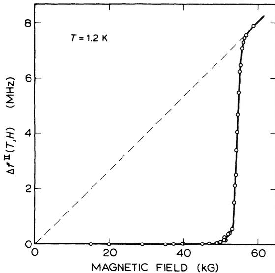
FIG. 5. Net magnetization at 1.2 K, as reflected in the NMR frequency of the in-layer  $^{19}\text{F}^{\text{II}}$  nuclei corrected for the Zeeman shift  $\Delta f^{\text{II}}(T, H)$  vs the magnetic field parallel to the  $c$  axis. The spin-flop transition is at  $54.5 \pm 0.5$  kG.
