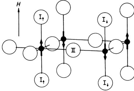
FIG. 1. Various  $F$  sites adjacent to the magnetic moments residing on the  $Mn^{2+}$  ions in the layer, with the magnetic field parallel to the tetragonal axis. The NMR frequencies of the out-of-layer  $^{19}F^{\uparrow}$  and  $^{19}F^{\downarrow}$  nuclei reflect the magnetizations of the up and down sublattices, respectively, while the NMR frequency of the in-layer  $^{19}F^{II}$  sites scales with the net magnetization.
