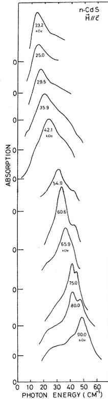
FIG. 1. Absorption spectra of the far-infrared cyclotron resonance in  $n$ -CdS ( $N_D - N_A = 7.1 \times 10^{15} \text{ cm}^{-3}$ ) at 19 K for magnetic fields from 23.2 to 90 kOe. The magnetic field direction is parallel to the  $c$  axis.
