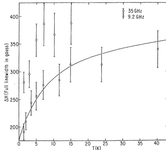
FIG. 6. Full TESR linewidth at half-maximum signal amplitude vs temperature for a 60-ppm Mg-Mn single crystal at a frequency of 9.2 and 35 GHz. The dc field orientation was set at  $\theta_c$ . The data have been corrected for the  $A/B$  line-shape factor. The solid line represents the relation appropriate to the bottlenecked limit, where the parameters  $\Delta H_{dl} = 175$  and  $\Delta H_{st} = 400$  G were chosen to fit the 9.2-GHz data.
