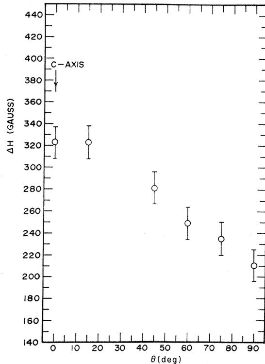
FIG. 4. Full linewidth at half-maximum signal amplitude versus magnet angle for pure Mg CESR. These data were obtained at  $T = 40^\circ\text{K}$  and spectrometer frequency 9.2 GHz. The sample foil was  $1.78 \times 10^{-3}$  cm thick, oriented with crystalline  $c$  axis perpendicular to the sample plane. Data have been corrected for the  $A/B$  line-shape factor.
