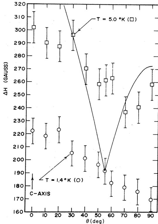
FIG. 3. TESR full linewidth at half-maximum signal amplitude vs magnet angle for Mg doped with 60-ppm (atomic) Mn. The spectrometer frequency was 9.2 GHz, and all data have been corrected for the  $A/B$  line-shape factor. The solid line on the figure reproduces a second-moment computation based on  $T = 1.4^\circ\text{K}$  and  $D_e = 69$  G. At  $0^\circ$  the field is normal to the sample and parallel to the  $C$  axis.
