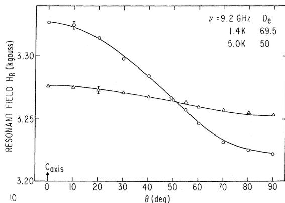
FIG. 2. Resonant field  $H_R$  vs magnet angle for a 60-ppm  $Mg$ - $Mn$  single-crystal sample at a frequency of 9.2 GHz. At  $0^\circ$  the field is normal to the sample and parallel to the  $C$  axis. The solid lines represent first-moment computations which determine the experimental value of the crystal-field-splitting parameter  $D_e$ .
