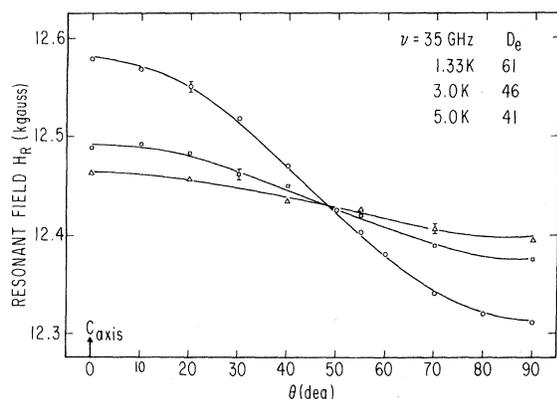
FIG. 1. Resonant field  $H_R$ , vs magnet angle for a 60-ppm  $Mg$ - $Mn$  single-crystal sample at a frequency of 35 GHz. At  $0^\circ$  the field is normal to the sample and parallel to the  $C$  axis. The solid lines represent first-moment computations which determine the experimental value of the crystal-field-splitting parameter  $D_e$ .
