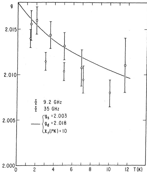
FIG. 5. TESR  $g$  value at  $\theta_c$  vs sample  $T$  for a 60-ppm Mg-Mn sample at a frequency of 9.2 and 35 GHz.  $\theta_c$  is that angle where the fine-structure lines coalesce. The solid line represents the relation appropriate to the bottlenecked limit where the values indicated were chosen to fit the 9.2-GHz data.
