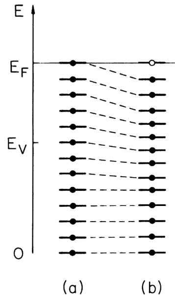
FIG. 4. When the ground state (a) is modified by the creation of a virtual level (b) the recoil profile has zero amplitude near threshold because an orbital occupied in the unperturbed system must be unoccupied in the perturbed configuration.
