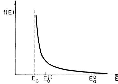
FIG. 6. Recoil spectrum for weak perturbations. The profile centers on the first-order perturbation energy  $E_0^{(1)}$  of the ground-state wave function when exposed to the perturbing potential, which must lie close to the threshold  $E_t$  when the perturbation is weak. However, the second moment shows that the spectrum spreads past the initial energy  $E_0^0$ , giving the line an asymmetrical shape.
