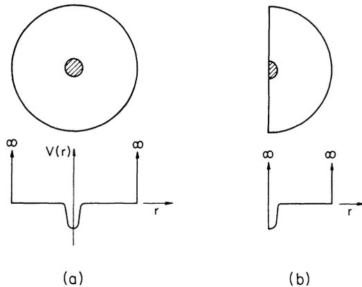
FIG. 1. Usual spherical model of a metal with a perturbation at its center may be modified as shown in (b) to give a model of surface absorption with no substantial change in the theory. A variety of alternative geometries are accessible.
