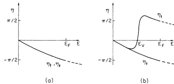
FIG. 2. (a) Phase shifts for spin-up and spin-down  $s$  waves at an empty cell screened only by  $s$  waves in a monovalent metal. (b) Same as (a) but with a full spin-up virtual level in the band at  $E_v$ ; this represents the excited configuration discussed in Sec. II A.
