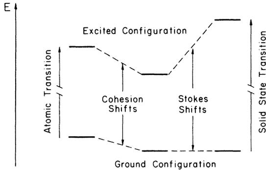
FIG. 5. Evolution of the threshold energy from the atomic-transition energy, through cohesion shifts of the ground- and excited-state energies and the excited-state Stokes shift.
