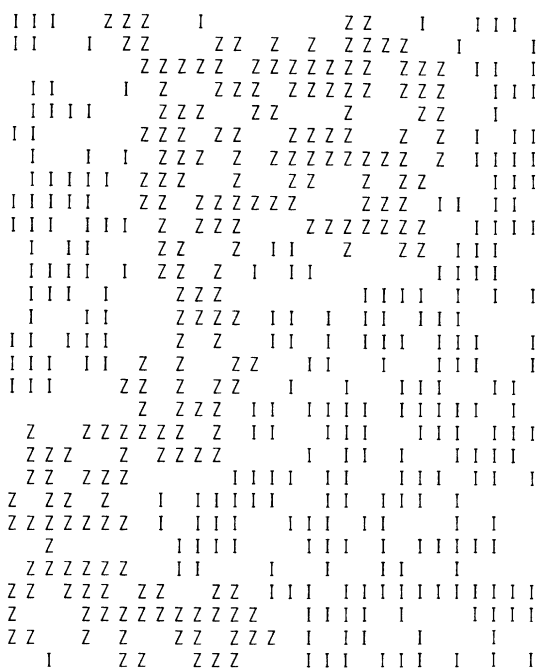
FIG. 5. A display of the cluster structure for the lattice given in Fig. 3. A Z denotes a site occupied by a molecule belonging to the largest A cluster. Other A clusters are represented by I's. The B molecules are denoted by blanks.
