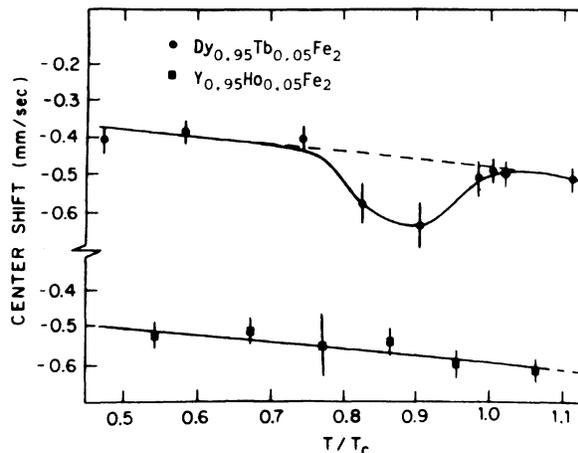
FIG. 3. The temperature dependence of the center of gravity of the Mössbauer spectra.
