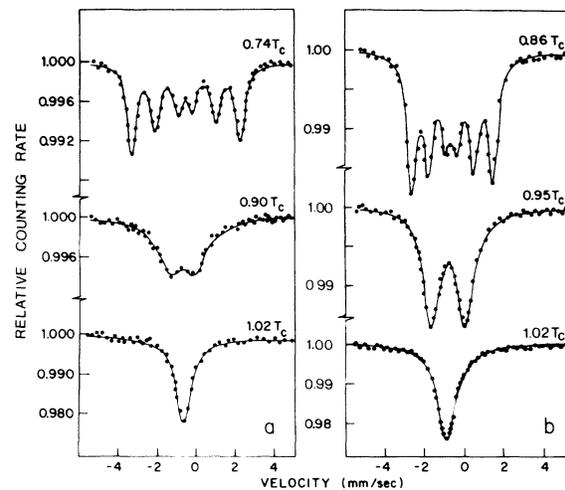
FIG. 1. Mössbauer spectra of  $^{57}\text{Fe}$  in  $\text{Dy}_{0.95}\text{Tb}_{0.05}\text{Fe}_2$  (26 mg/cm<sup>2</sup>) (a), and  $\text{Y}_{0.95}\text{Ho}_{0.05}\text{Fe}_2$  (31 mg/cm<sup>2</sup>) (b). The solid curves represent theoretical best fit spectra composed of six Lorentzian absorption lines.
