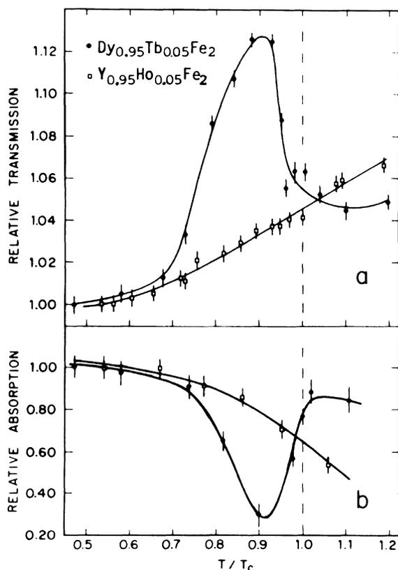
FIG. 2. (a) The transmitted intensity (normalized to room-temperature transmission) as a function of temperature. (b) The temperature dependence of the area under the Mössbauer absorption spectra, normalized to the area at room temperature.
