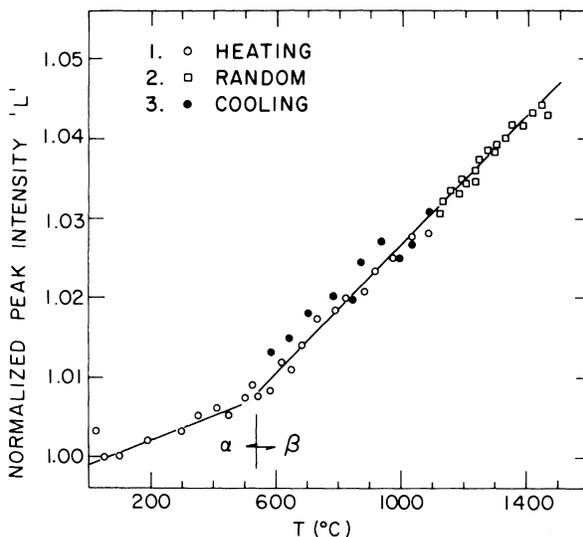
FIG. 2. Temperature dependence of the line-shape parameter  $L$ , describing the Doppler-broadened line-width of annihilation photons from a  $^{68}\text{Ge}$  source in  $\text{Zr}_{0.53}\text{Ti}_{0.47}$ . Data labeled "random" were not accumulated in any regular sequence—otherwise the numbering and labeling in the legend have a meaning as in the Fig. 1 caption.
