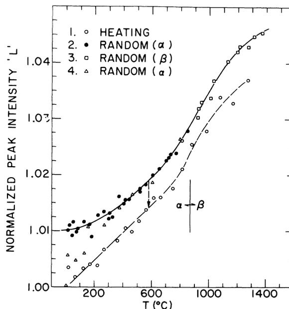
FIG. 3. Temperature dependence of the line-shape parameter  $L$ , describing the Doppler-broadened line-width of annihilation photons from a  $^{68}\text{Ge}$  source in Zr. Numbering and labeling have the sense described in the captions for Figs. 1 and 2. Data 1 coincide with data 2 and 4 in the vicinity of 600 °C, but they have been displaced downwards by 2.0 scale divisions for ease of viewing.
