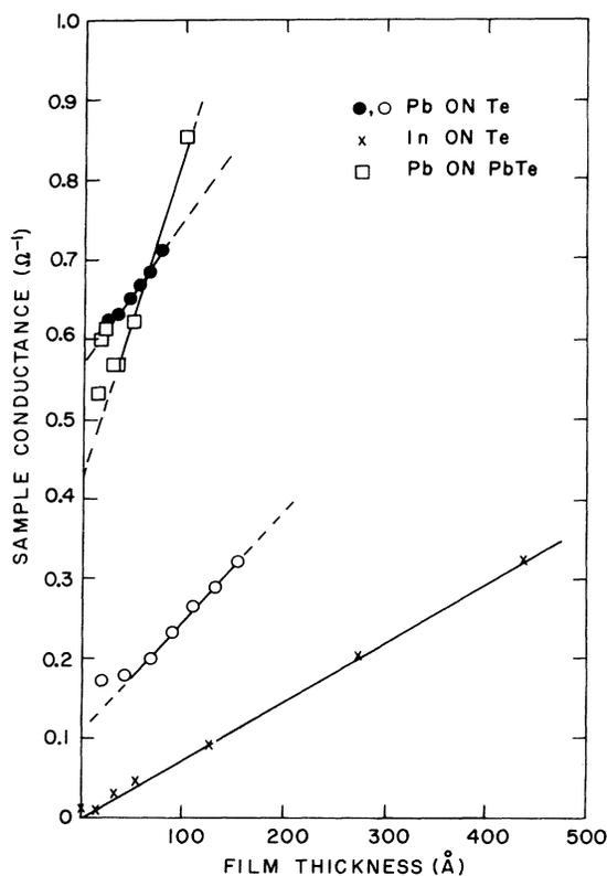
FIG. 1. Sample conductance as a function of metal-film thickness for samples consisting of Pb deposited on PbTe, Pb deposited on Te, and In deposited on Te. Film resistivity was obtained from the approximately linear regions of the data.
