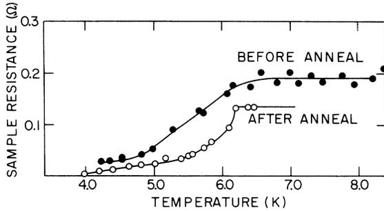
FIG. 3. Resistance as a function of temperature for a sample consisting of In deposited on PbTe at about 7 K, before and after annealing to room temperature by allowing the cryostat to warm overnight.
