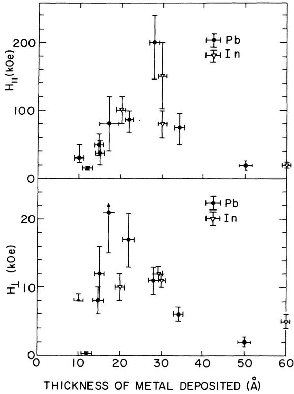
FIG. 6. Critical fields parallel ( $H_{c||}$ ) and perpendicular ( $H_{c\perp}$ ) to the plane of the substrate surface, for Pb and In films deposited on PbTe at 77 K, as a function of the thickness of metal deposited. The films were warmed to room temperature and exposed to air in being transferred to a Dewar for measurement. Neither  $H_{c||}$  nor  $H_{c\perp}$  increases with decreasing thickness below about 20–30 Å, as expected for a continuous film.
