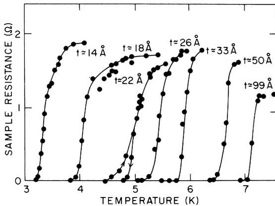
FIG. 4. Resistance of a sample consisting of Pb deposited on PbTe at about 77 K, as a function of temperature, for several thicknesses of deposited Pb films. The measurements were made *in situ*, without warming about 80 K (except for an accidental warming to about 115 K between  $t = 22$  Å and  $t = 26$  Å).
