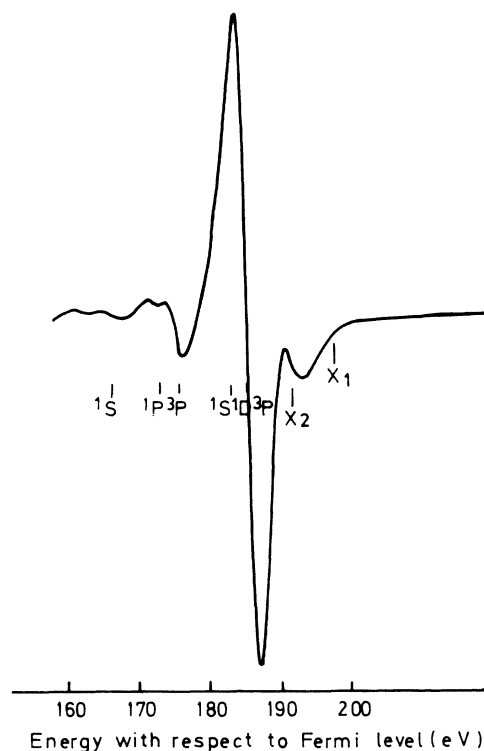
FIG. 6. L_{23}VV Auger spectrum of chlorine adsorbed on Cu(100) in the dN/dE mode. See Fig. 1 caption.
