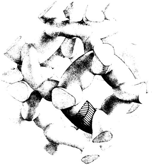
FIG. 7. Portion of the third-zone electron surface of lead showing the location of the section depicted in Fig. 3. Modified from, M. Ya. Azbel, M. I. Kaganov, and L. M. Lifshitz, Conduction Electrons in Metals (Freeman, San Francisco, 1973), Copyright © 1973 by Scientific American, Inc. All rights reserved.
