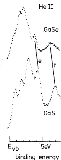
FIG. 7. Comparison of the He II energy distributions for GaSe and GaS. Note the shift of bands c to f to higher binding energy in the sulphide with consequent increase in total bandwidth. Peaks e and f maintain constant separation for both materials.
