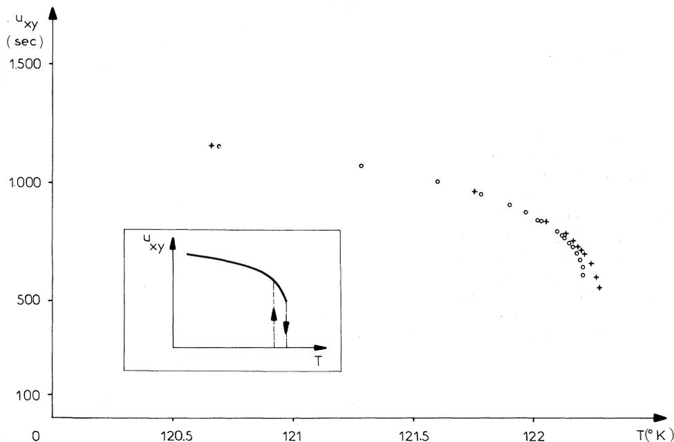
FIG. 3. Temperature dependence of the spontaneous shear. The points are related to decreasing temperature; the crosses represent increasing temperature. The usual thermodynamic behavior is shown on the left.
