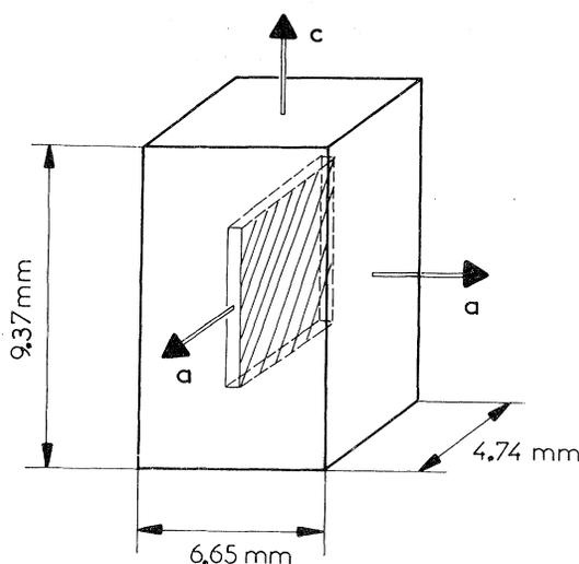
FIG. 1. Dimension and orientation of the sample; the investigated volume element is sketched by dotted lines.
