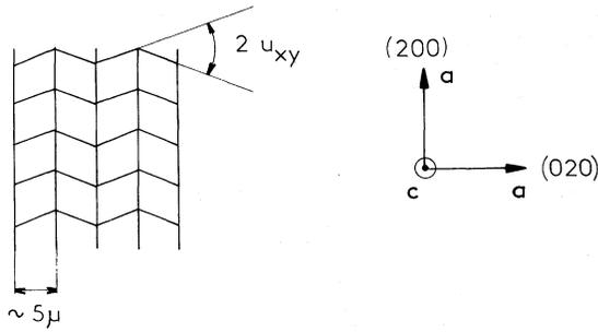
FIG. 2. Domain structure in the ferroelectric phase;  $u_{xy}$  is the shear angle.
