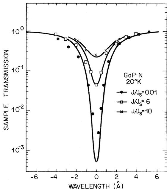
FIG. 3. Sample transmission spectrum at three different intensities. "0" on the horizontal scale corresponds to 5349.0 Å. The points are experimental; the solid curves are theoretical, as discussed in the text.
