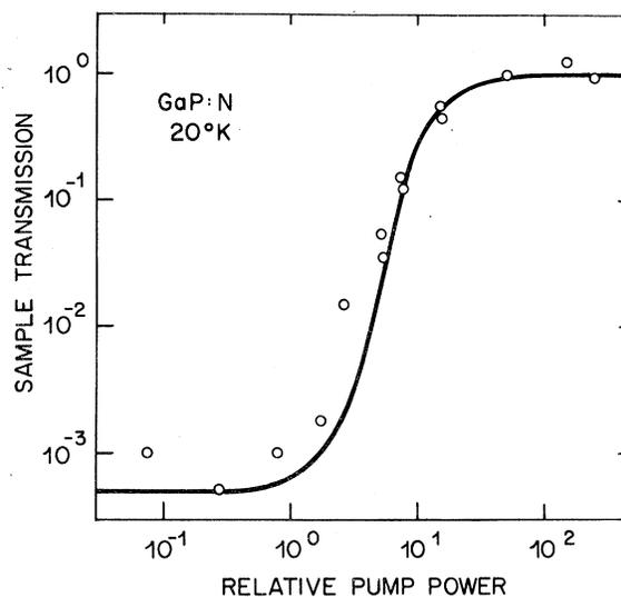
FIG. 4. Sample transmission vs incident pump power. The points are experimental and the solid curve is theoretical [Eq. (1)]. The highest pump power (last experimental point) was  $\approx 200$  W focused into  $\sim 30$ - $\mu$ m diameter spot.  $J_{\max} = 2.5 \times 10^{17}$  photons/cm<sup>2</sup>. The theoretical curve is plotted for  $J_s = 10^{15}$  photons/cm<sup>2</sup>.
