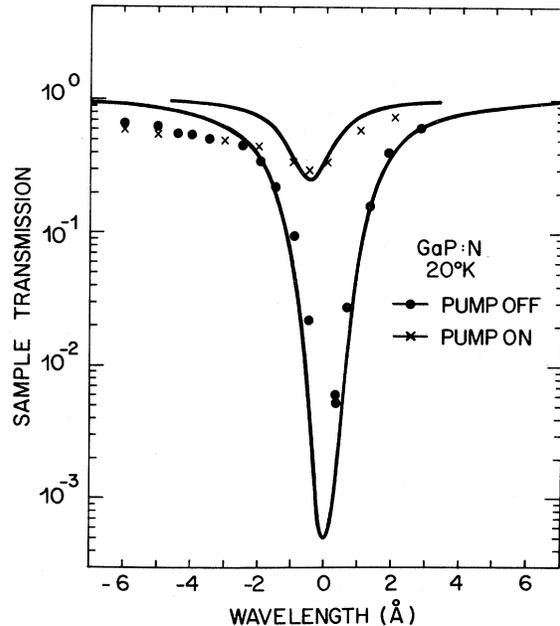
FIG. 5. Transmission spectrum near the A line obtained with the probe beam for the pump beam on and off. The pump beam was at  $4880 \text{ \AA}$ .
