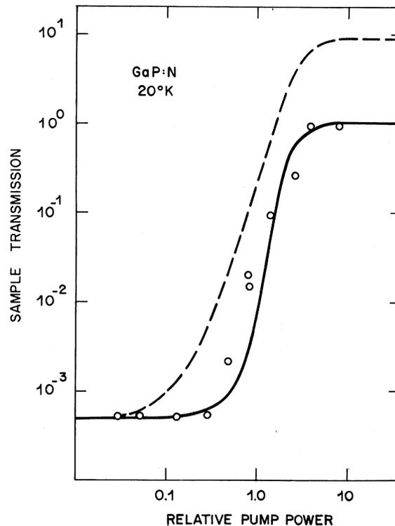
FIG. 6. Sample transmission vs pump power. The last experimental point corresponds to  $\approx 500$  W focused into  $30\text{-}\mu\text{m}$  diameter spot.
