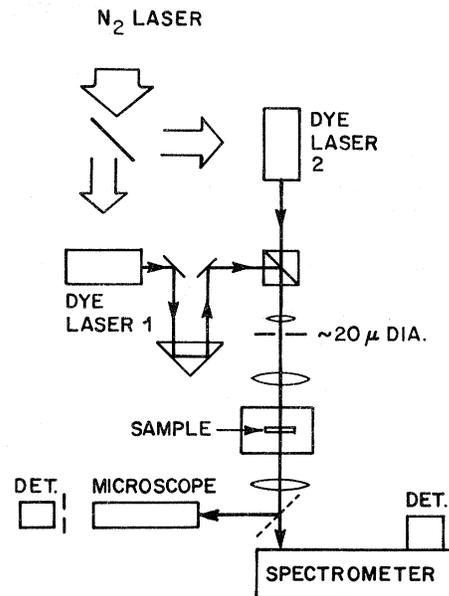
FIG. 2. Schematic diagram of experimental arrangement.
