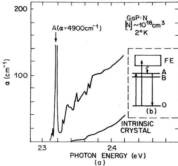
FIG. 1. Absorption spectrum of GaP in the vicinity of the A line for an intrinsic crystal (no N doping) and for a crystal doped with  $\sim 10^{18}$  N/cm<sup>3</sup> [P. J. Dean, J. Lumin. **1**, 2, 407 (1970)]. The inset shows the energy-level scheme relevant to this paper.
