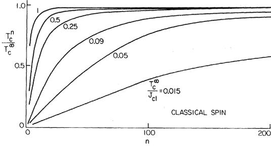
FIG. 1.  $T_c^n/T_c^\infty$  as a function of  $n$  for several values of  $T_c^\infty/J_{c1}$  ( $k_B=1$ ) for the classical spin model.
