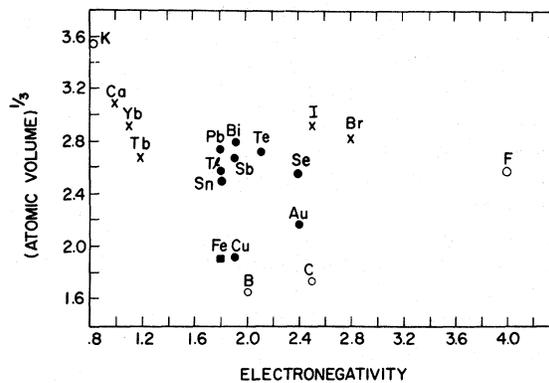
FIG. 7. Darken-Gurry plot for impurities implanted into Fe at room temperature. The atomic volume is in arbitrary units and the electronegativity follows Pauling's scale. ●, >80% substitutional; ×, 50-80% substitutional; ○, <50% substitutional.
