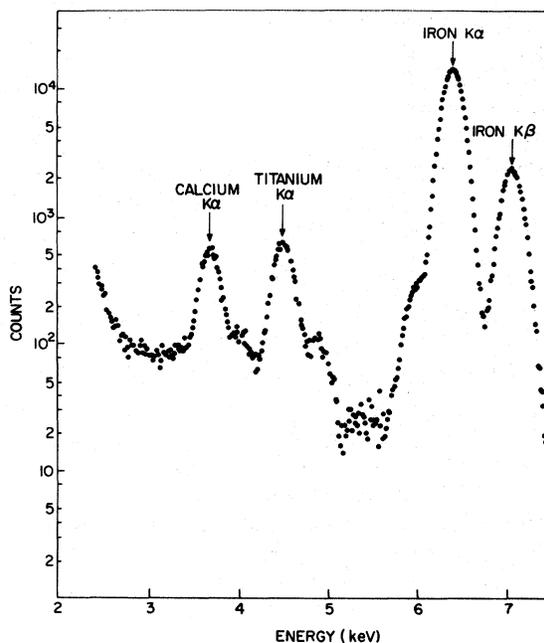
FIG. 1. X-ray spectrum obtained by bombardment of a calcium-implanted iron single crystal with 1.5-MeV  $^4\text{He}^+$  ions incident in a  $\langle 111 \rangle$  axial channeling direction. The total implant dose was approximately  $3 \times 10^{15} \text{ cm}^{-2}$ .
