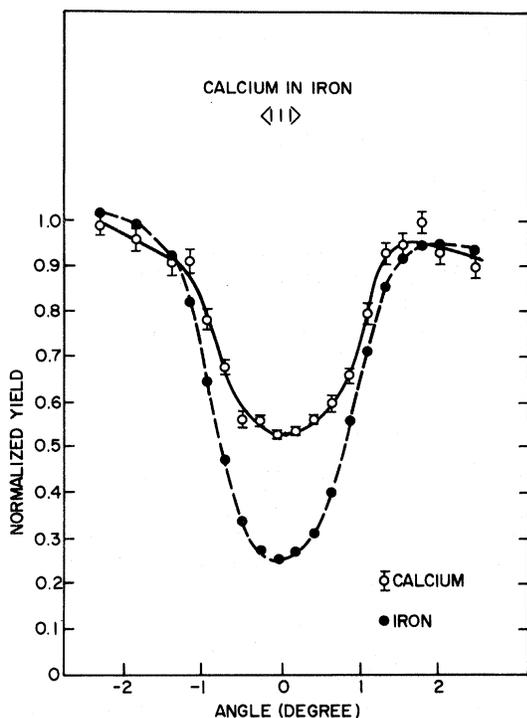
FIG. 2. Angular scan across the  $\langle 111 \rangle$  axis in a calcium-implanted iron single crystal.
