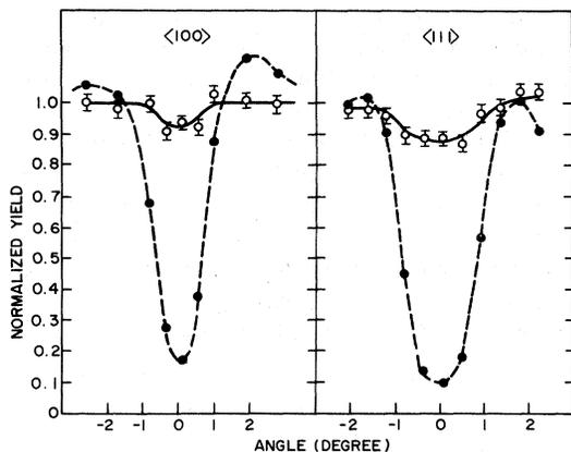
FIG. 5. Potassium in iron angular scans.
