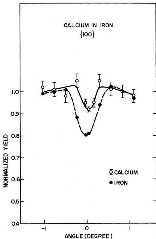
FIG. 4. Calcium in iron {100} angular scan.
