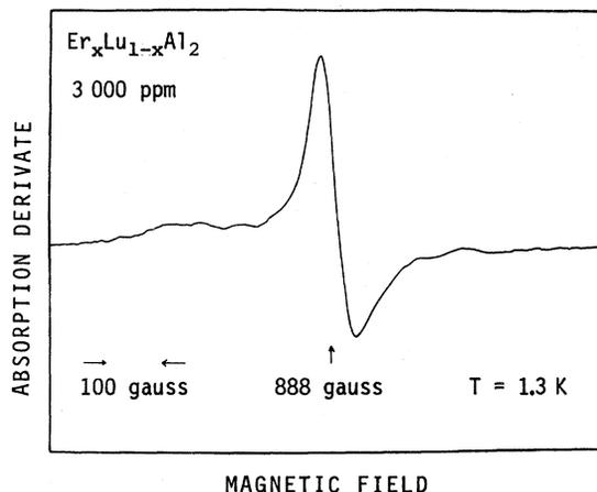
FIG. 3. EPR spectra of Er in  $\text{LuAl}_2$  at 1.3 K. The Er concentration is 3000 ppm.
