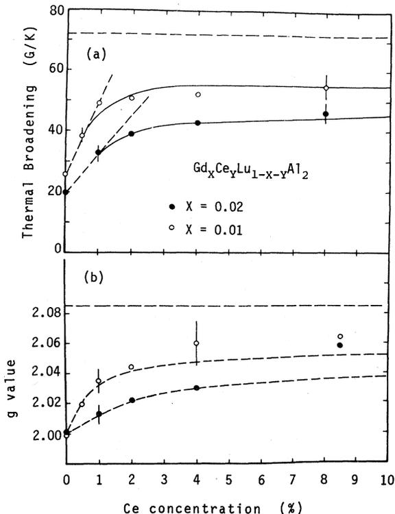
FIG. 2. High-temperature (a) thermal broadening,  $\Delta H/T$ , and (b)  $g$  value of  $\text{Gd}_x\text{Ce}_y\text{Lu}_{1-x-y}\text{Al}_2$  ( $x=0.02, 0.01$ ) as a function of Ce concentration. The horizontal dashed lines represent the unbottlenecked values of  $\Delta H/T$  and  $g$ .
