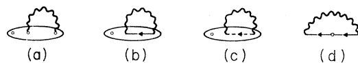
FIG. 7. First-order-correction diagrams in the calculation of the population of molecular-field state |1\rangle . Small circles that are not connected to the interaction lines are the L_{11} vertices; those which attach to interaction lines are the L_{11}-L_{II}-\langle S^z \rangle vertices.
