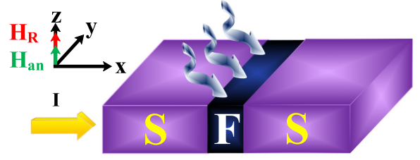
FIG. 1. Schematic diagram depicting \varphi_0 under the influence of external electromagnetic radiation. The magnetic field component ( H_R ), and the anisotropic field ( H_{an} ) are in z direction, while the bias current I is along the x direction.
