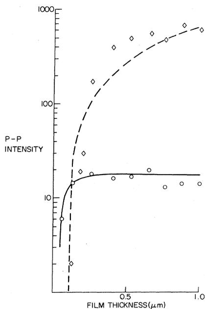
FIG. 12. Variation of the peak-to-peak intensity with film thickness for a bulk spin wave ( $\diamond$ ) and the surface spin wave ( $\circ$ ). (Ref. 1.)
