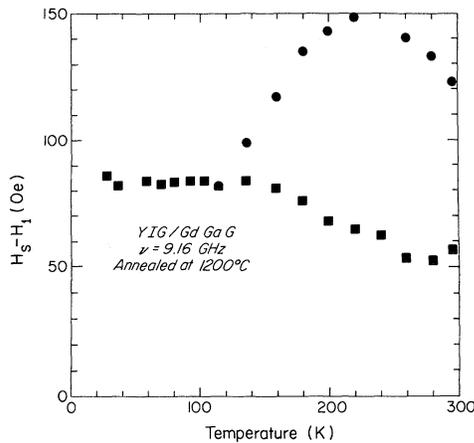
FIG. 17. Separation of the first body mode and first and second surface modes, respectively, as a function of temperature for a YIG film.
