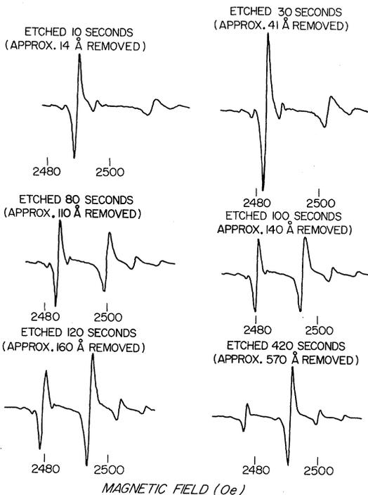
FIG. 14. Traces of the second and third high-field spin-wave modes as the film thickness is decreased by etching for a YIG film having two surface modes.
