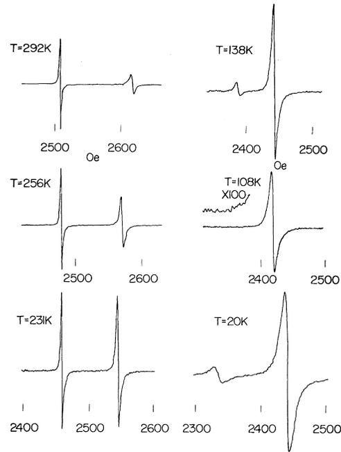
FIG. 15. Traces of the first two high-field spin-wave modes as a function of temperature for a YIG film having a single surface mode at room temperature.
