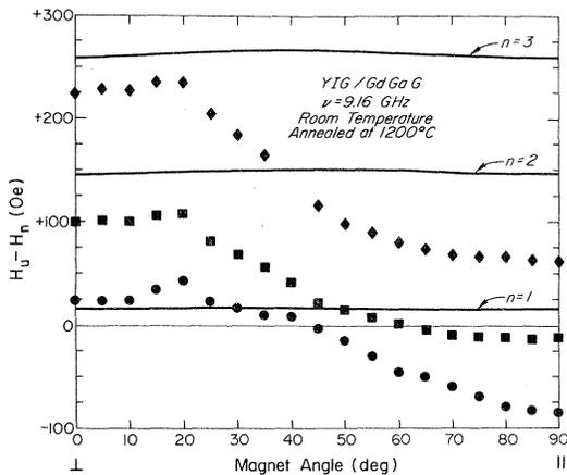
FIG. 10. Angle dependence of the magnetic field separation of the observed positions of the spin-wave modes  $H_n$  from the calculated position of the uniform mode  $H_u$  for a typical YIG film having two surface modes.
