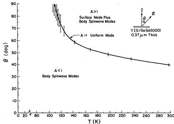
FIG. 16. Temperature dependence of the critical angle for a YIG film.
