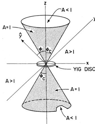
FIG. 3. Angle dependence of the surface parameter  $A$  for a tensorial surface anisotropy energy.
