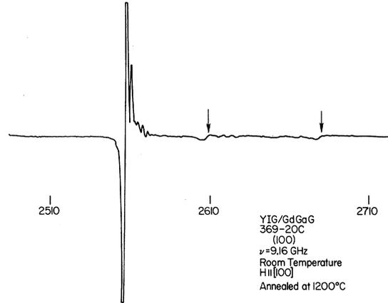
FIG. 9. Trace of the high-field modes observed at parallel resonance, 9.2 GHz, and room temperature for a YIG film annealed at  $1200^\circ\text{C}$  in an oxygen atmosphere for 6 h.
