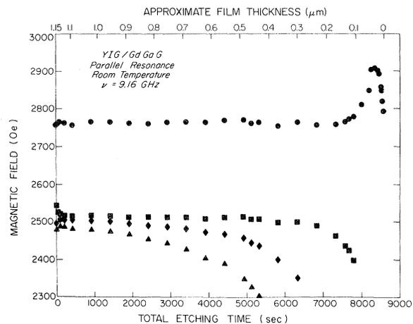
FIG. 13. Effect of etching on the resonant-field position of the high-field spin-wave modes for a YIG film having two surface modes.
