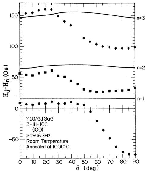
FIG. 8. Angle dependence of the magnetic field separation of the observed positions of the spin-wave modes  $H_n$  from the calculated position of the uniform mode  $H_u$  for a typical YIG film having a single surface mode.
