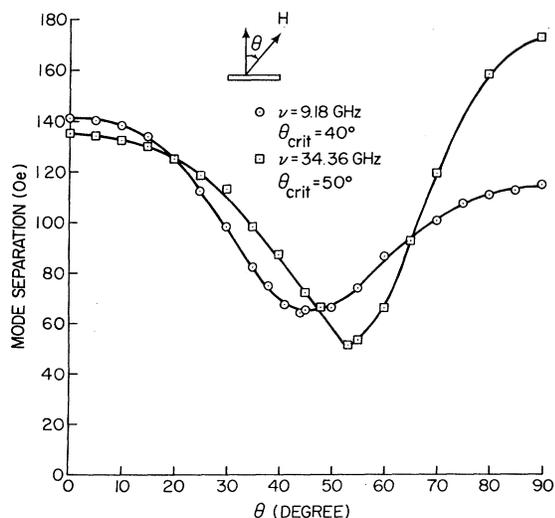
FIG. 6. Angle dependence of the resonant-field separation between the two highest field modes at 9.2 and 34.4 GHz and room temperature for a typical YIG film having a single surface mode.
