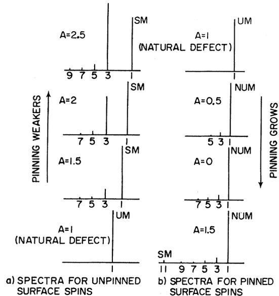
FIG. 2. SWR spectra calculated for various values of the surface parameter  $A$ , i.e., for various pinning of the surface spins. The film has 11 spin layers. UM denotes a uniform mode, SM a surface mode, NUM a nonuniform body mode.
