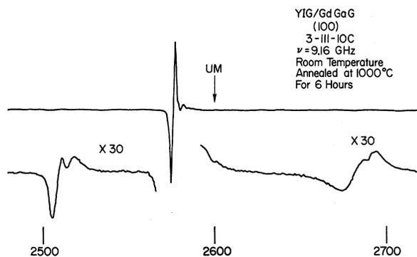
FIG. 4. Trace of the high-field modes at parallel resonance, 9.2 GHz and room temperature for a YIG film annealed at 1000°C in an oxygen atmosphere for 6 h.
