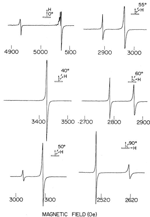
FIG. 5. Trace of the first two modes observed at six orientations at 9.2 GHz and room temperature for a typical YIG film having a single surface mode.
