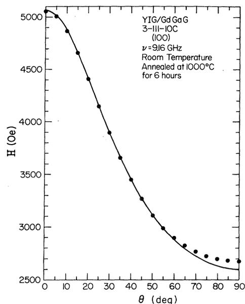
FIG. 7. Angle dependence of the resonant-field position of the highest field mode of a typical YIG film having a single surface mode.
