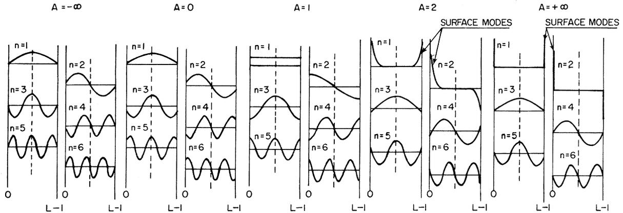
FIG. 1. Shapes of spin-wave modes (with low  $n$ ) for various values of the surface parameter  $A$ . Symmetric and anti-symmetric modes correspond to odd and even  $n$ , respectively.
