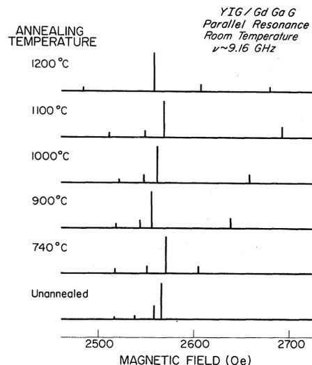
FIG. 11. Stick diagrams representing the parallel resonance spectra of a series of YIG films showing the effect of annealing on the resonant-field position of the spin-wave modes.
