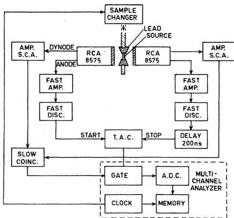
FIG. 2. Block diagram of the electronics used to measure the influence of the chemical environment on the decay constant of the 24-keV  $\gamma$  transition of <sup>119</sup>Sn.
