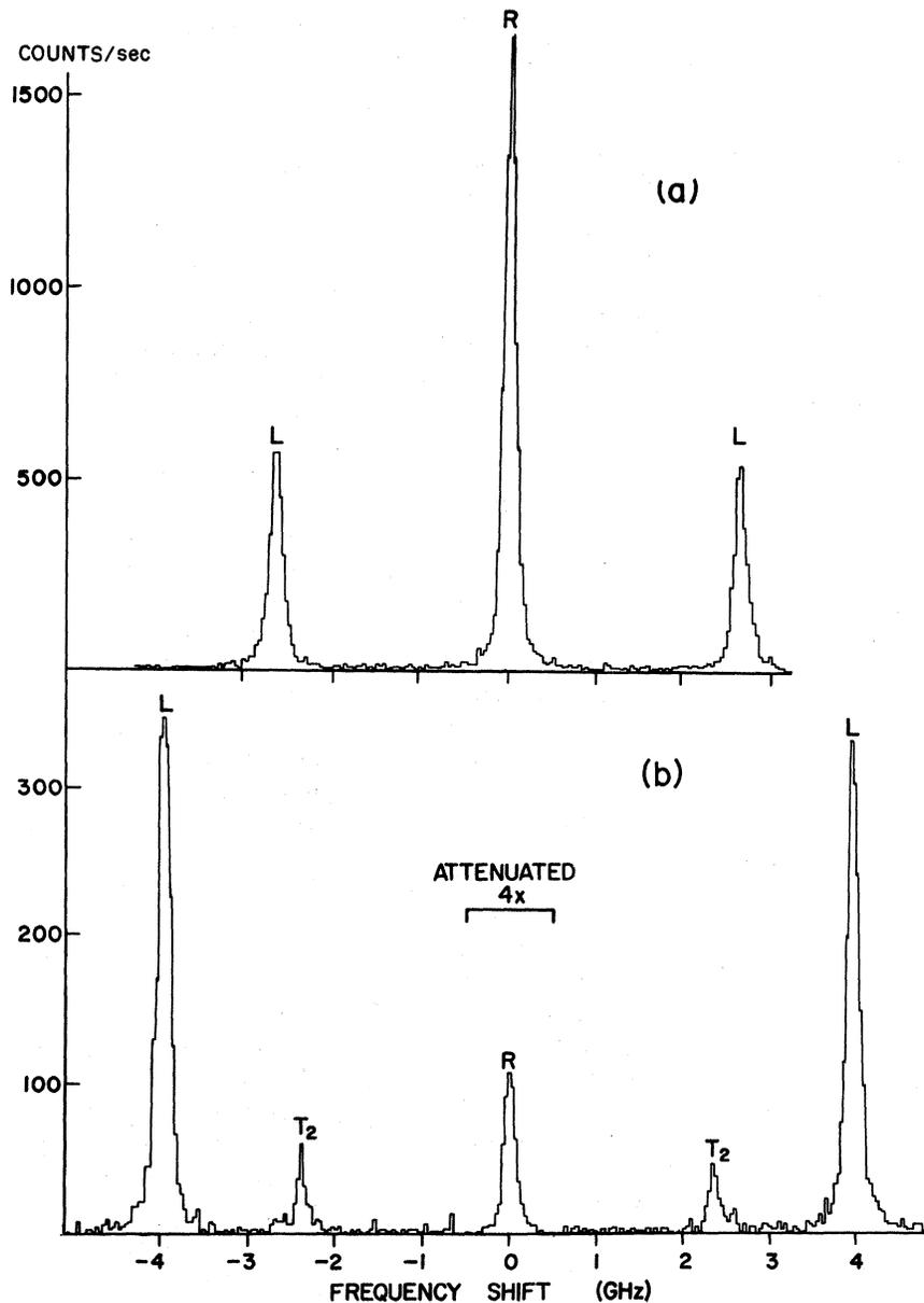
FIG. 1. Typical Brillouin spectra of (a) liquid, and (b) solid krypton.
