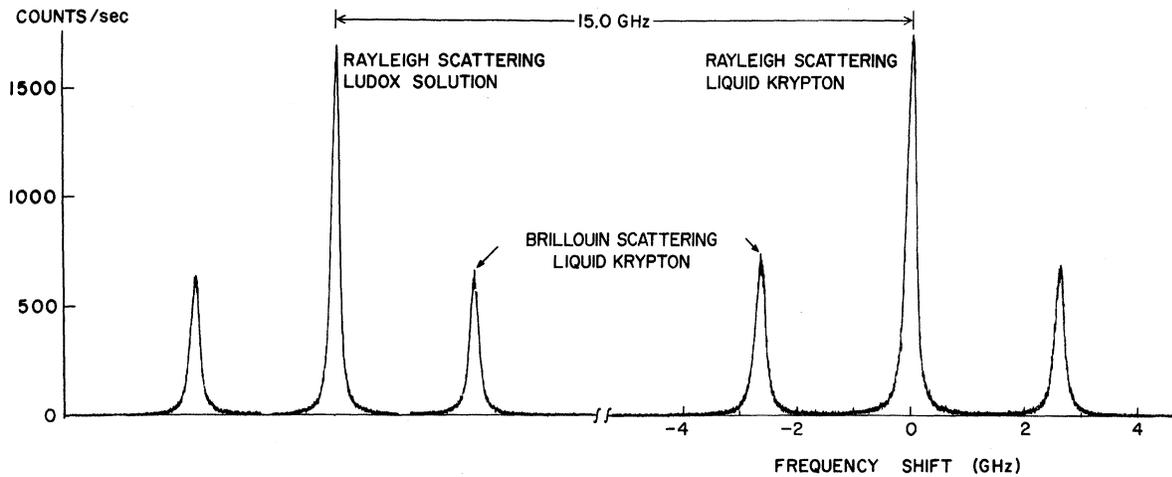
FIG. 3. Typical scan for measuring the relative intensity of Brillouin components of krypton to the Rayleigh scattering from Ludox solution. From left to right the components are  $B_K$ ,  $R_L$ ,  $B_K$ ,  $B_K$ ,  $R_K$ ,  $B_K$  (where  $B_K$  represents Brillouin component from krypton, and  $R_L$  and  $R_K$  represent Rayleigh scattering from Ludox and krypton, respectively).
