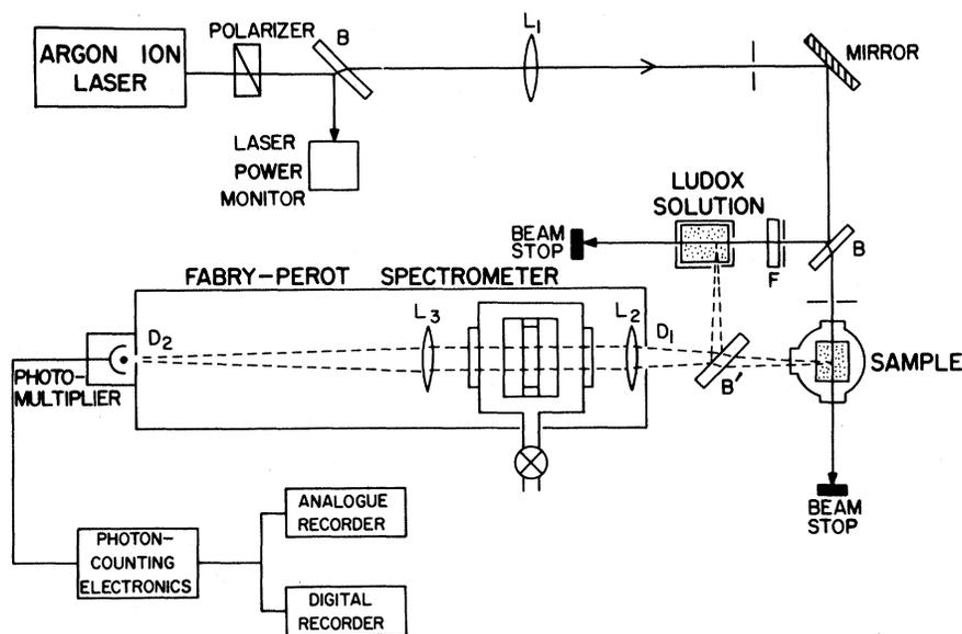
FIG. 2. Schematic diagram of apparatus for intensity measurements of liquids using a Ludox solution as intensity standard.
