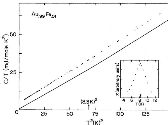
FIG. 3. Specific heat of  $\text{Au}_{0.99}\text{Fe}_{0.01}$  in the temperature region 2–12 K is shown as a plot of  $C/T$  vs  $T^2$ . The solid curve is the calculated nonmagnetic contribution to the specific heat of the alloy. The insert shows the ac susceptibility results of the same sample.
