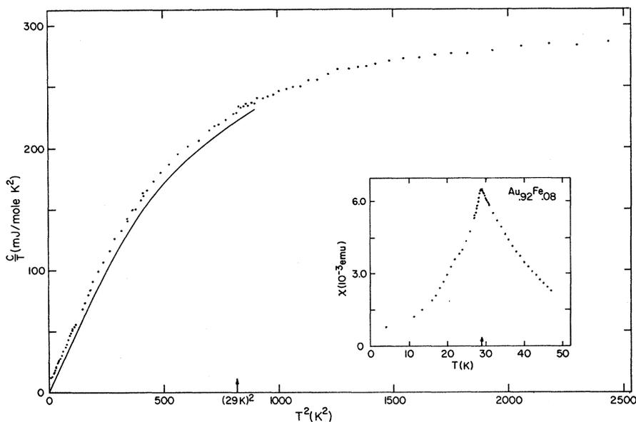
FIG. 2. Specific heat of  $\text{Au}_{0.92}\text{Fe}_{0.08}$  in the temperature region 3–50 K is shown as a plot of  $C/T$  vs  $T^2$ . The solid curve is the calculated nonmagnetic contribution to the specific heat of the alloy between 0 and 30 K. The insert shows the susceptibility results of the same sample, which were provided by S. A. Werner.
