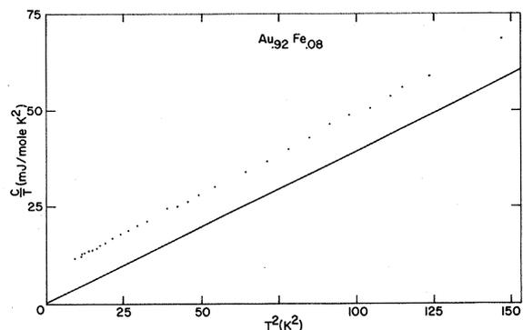
FIG. 1. Specific heat of  $\text{Au}_{0.92}\text{Fe}_{0.08}$  in the low-temperature region is shown as a plot of  $C/T$  vs  $T^2$ . The solid curve is the calculated nonmagnetic contribution to the specific heat of the alloy.
