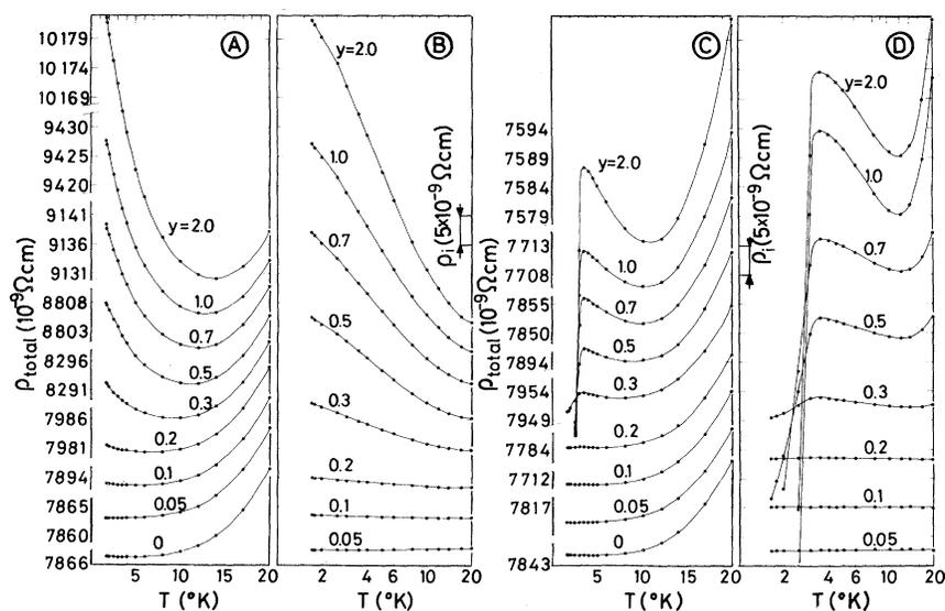
FIG. 8. As in Fig. 7 but for samples  $(\text{Au}_{36}\text{Ag}_{70})_{100-y}\text{Yb}_y$ : (A and B) are as-cast; (C and D) annealed for 1 h at 560°C, after cooled working.
