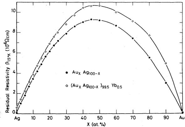
FIG. 3. Concentration dependence of the residual resistivity of the (AuAg) Yb alloys and their corresponding (AuAg) hosts.
