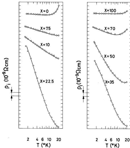
FIG. 5. Logarithmic temperature dependence of the impurity resistivity  $\rho_i$ , found for the alloys of Fig. 4.
