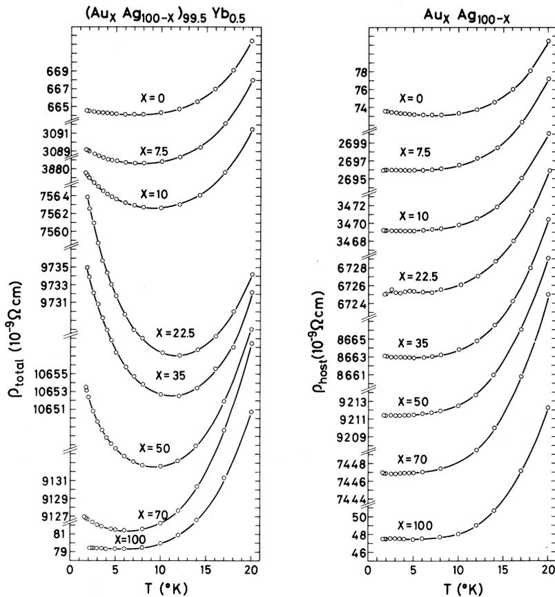
FIG. 4. Temperature dependence of the resistivities of some representative (AuAg) Yb alloys and their corresponding AuAg hosts.
