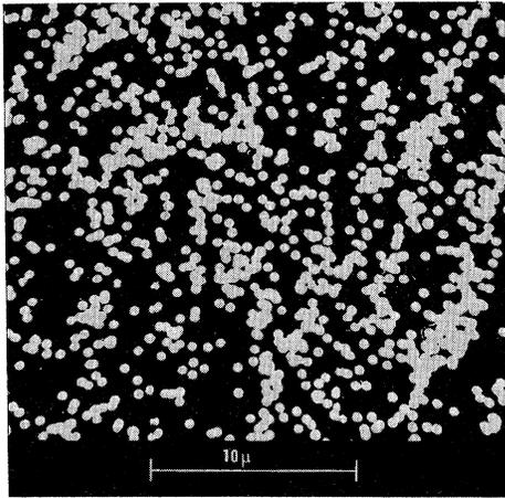
FIG. 9. Surface topography obtained by microprobe analysis of the  $(\text{Au}_{30}\text{Ag}_{70})_{93}\text{Yb}_2$  sample after homogenization for 1 week at  $560^\circ\text{C}$ . The clear points represent the zones containing the intermetallic compound  $\text{YbAu}_3$ .
