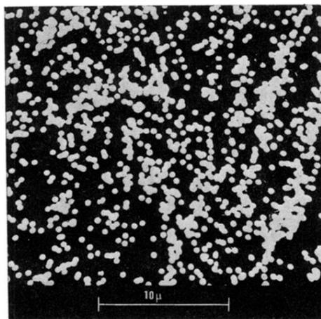
FIG. 9. Surface topography obtained by microprobe analysis of the  $(\text{Au}_{30}\text{Ag}_{70})_{98}\text{Yb}_2$  sample after homogenization for 1 week at 560 °C. The clear points represent the zones containing the intermetallic compound  $\text{YbAu}_3$ .
