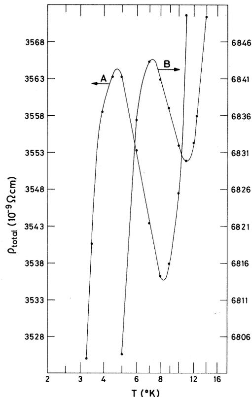
FIG. 10. Logarithmic temperature dependence of the resistivity of the Yb-Au intermetallic compounds. (a)  $\text{YbAu}_3$  (+  $\text{YbAu}_4$ ); (b)  $\text{YbAu}$  (+  $\text{YbAu}_2$ ).
