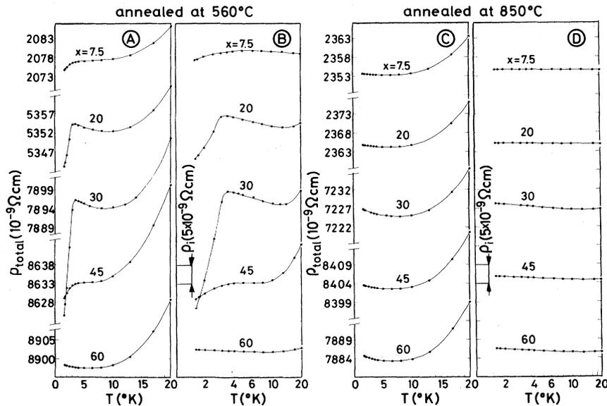
FIG. 7. Temperature dependence of the total resistivity  $\rho_{\text{tot}}(T)$ , and Yb contribution  $\rho_i(\ln T)$ , of  $(\text{Au}_x\text{Ag}_{100-x}\text{Yb}_{0.5})$  (nominal concentration) obtained after annealing the samples for 1 h, after cooled working: (A and B)  $560^\circ\text{C}$ ; (C and D)  $850^\circ\text{C}$ .
