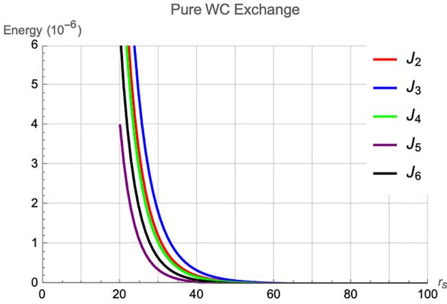
FIG. 5. Exchange coefficients of the pure WC (in units of the Hartree energy  $e^2/4\pi\epsilon a_B$ ) as a function of  $r_s$ , calculated from the semiclassical expression (16). The processes corresponding to  $J_2, \dots, J_6$  are schematically illustrated in Fig. 4(a). Within the WC phase ( $r_s \gtrsim 30$ ), the instanton approximation is well-justified for the calculation of these ring-exchange processes since  $\sqrt{r_s} S_a \gg 1$ .
