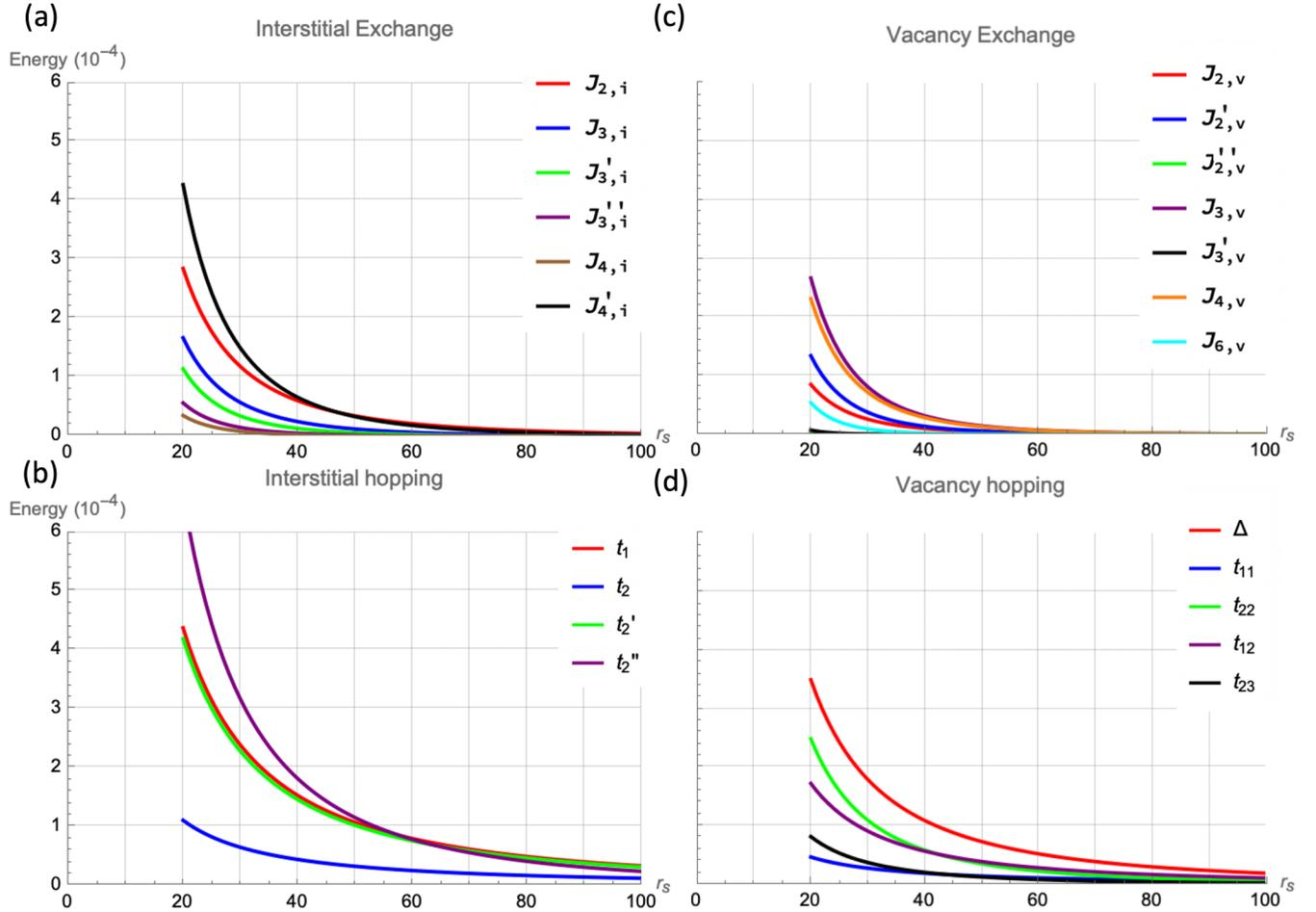
FIG. 6. Hopping matrix elements and exchange coefficients involving a defect (in units of  $e^2/4\pi\epsilon a_B$ ) within the semiclassical approximation. Note that the y-axis scale here is a factor of 100 larger than in Fig. 5. Hence, the dynamical processes involving an interstitial or a vacancy have much larger energy scales than the exchange processes in the pure WC.
