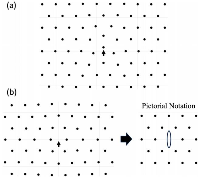
FIG. 2. (a) A classical centered interstitial and (b) a vacancy configuration. Small black arrows are drawn to indicate the positions of the interstitial [panel (a)] and the vacancy [left panel of (b)]. The vacancy configuration has  $D_2$  symmetry, and not the full  $D_6$  symmetry of the underlying WC; therefore, a vacancy has three possible orientations  $\alpha$ . We introduce a pictorial notation for the vacancy for later convenience.
