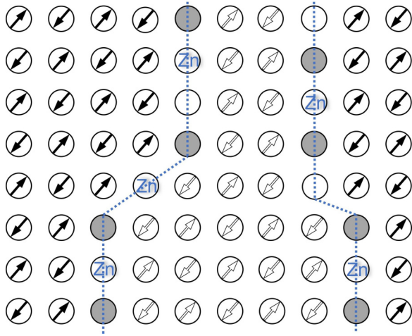
FIG. 1. A schematic drawing of parallel stripe order in the La214 cuprate with quenched nonmagnetic Zn impurities replacing Cu in the \text{CuO}_2 plane. Only the Cu sites are shown. This 2D parallel stripe structure is an inhomogeneous arrangement of holes (solid gray circles), and spins (arrows) within a \text{CuO}_2 plane, while the open circles represent paramagnetic sites. Shading of the arrowheads distinguishes the antiphase Néel domains.
