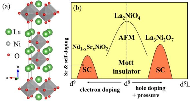
FIG. 1. (a) Crystal structures of an idealized bilayer perovskite, represented using the program VESTA [33]. (b) Schematic suggested phase diagram of nickelates based on electron doping from  $d^8$  to  $d^9$  and hole doping from  $d^8$  to  $d^{8L}$ . The electron concentration per Ni of  $\text{Nd}_{1-x}\text{Sr}_x\text{NiO}_2$  is reduced from  $d^9$  due to Sr doping and partial charge transfer (self-doping) from Ni to Nd [7–9].
