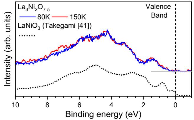
FIG. 4. HAXPES valence band spectra of polycrystalline  $\text{La}_3\text{Ni}_2\text{O}_{7-\delta}$  measured at 80 K (blue line) and at 150 K (red line), together with that of LaNiO<sub>3</sub> (dotted line) from Ref. [41].
