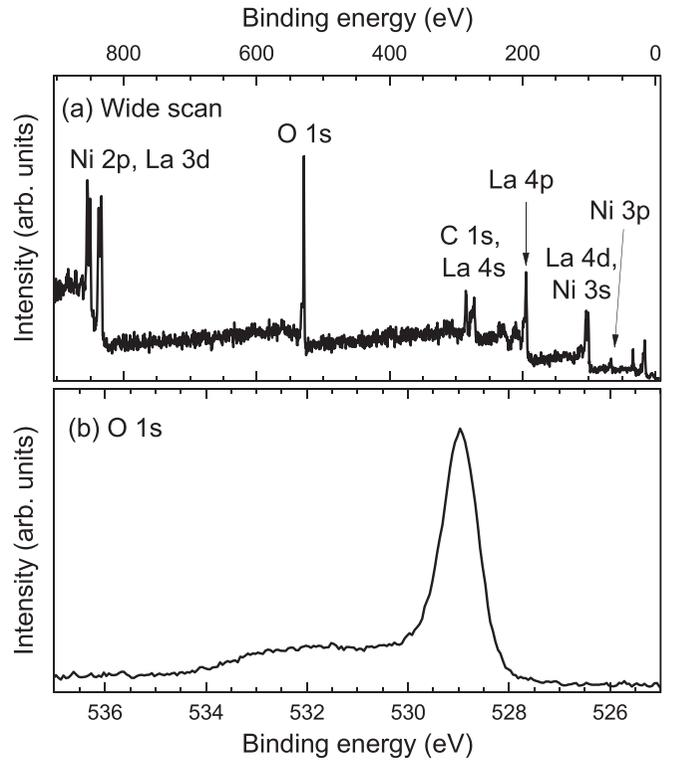
FIG. 2. (a) Wide scan and (b) O  $1s$  core level spectra of the polycrystalline  $\text{La}_3\text{Ni}_2\text{O}_{7-\delta}$ .
