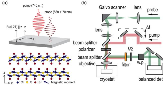
FIG. 1. Experimental setup for MOKE imaging. (a) Crystal structure of CrSBr and experimental geometry. The blue arrows represent the magnetic moments which are slightly canted away from the easy  $b$  axis in the external magnetic field. (b) Optical setup of the tr-MOKE imaging system. In all experiments, the sample temperature is 5 K and the external field is 0.2 T along  $z$ .
