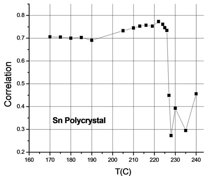
FIG. 7. Maximum value of the spatial correlation between two speckle patterns separated in time by 120 s, as a function of temperature, for laser light reflected from the surface of a  $\beta$ -Sn polycrystal. We identify the dip between 226 °C and 230 °C as due to grain-boundary melting.
