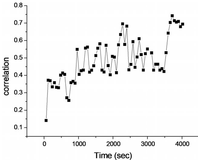
FIG. 9. Time dependence of the correlation of the speckle pattern over successive 60-s intervals during grain-boundary melting inside a 1.4-mm-thick polycrystalline Sn sample maintained at 229 °C. The high correlation after 3500 s indicates that all the grain boundaries in this sample have melted.
