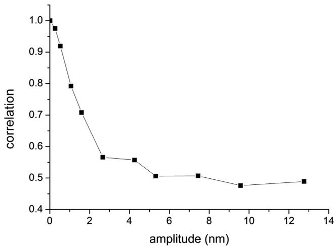
FIG. 2. Maximal correlation between two simulated laser speckle patterns at  $\lambda = 532$  nm, scattered by an arbitrary substrate undergoing random height fluctuations of amplitude  $d$ .
