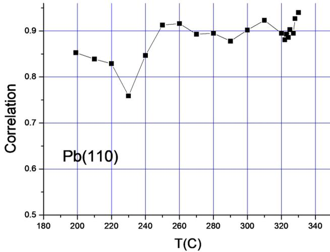
FIG. 4. Temperature dependence of the maximum correlation between speckles of light scattered from a Pb(110) surface. The time interval between the correlated images is 120 s. The dip at 230 °C is interpreted as the onset of surface melting, in agreement with [6] and [7].
