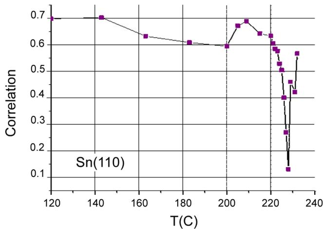
FIG. 6. Maximum value of the spatial correlation between two speckle patterns separated in time by 120 s, as a function of temperature, for laser light reflected from the (110) surface of a  $\beta$ -Sn crystal. We identify the dip between 140 °C and 210 °C as due to surface melting and that between 224 °C and 229 °C as due to grain-boundary melting.
