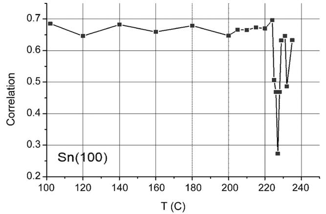
FIG. 5. Maximum value of the correlation between two speckle patterns separated in time by 120 s, as a function of temperature, for a (100) surface of a  $\beta$ -Sn crystal ( $T_M = 231.8^\circ\text{C}$ ). We identify the dip between 224 °C and 229 °C as due to grain-boundary melting and that at 232 °C as bulk melting.
