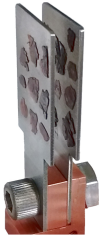
FIG. 8. KYbSe 2 sample used to measure the field-dependent spin excitations on CNCS. Nineteen platelike crystals were coaligned and glued to two aluminum plates with the [110] direction vertical and the [001] direction orthogonal to the aluminum surface.
