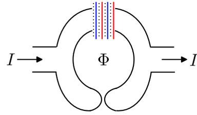
FIG. 4. SQUID geometry to measure the negative interlayer Josephson coupling. For an even number of layers, the SQUID enclosed a  $\pi$  flux
