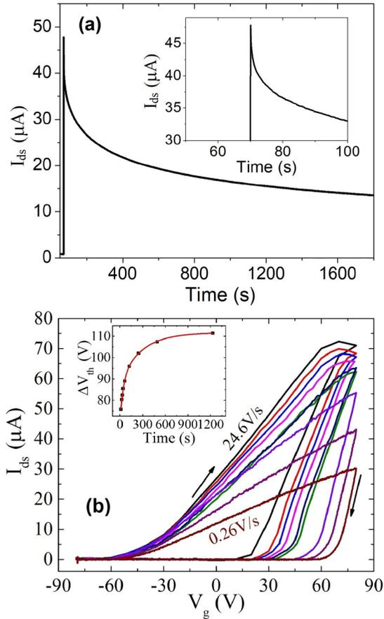
FIG. 4. (a) The measured time dependence of  $I_{ds}$  when  $V_g$  is changed abruptly from  $-80$  to  $+80$  V at  $t = 70$  s. The inset shows the zoomed-in initial part of the relaxation. (b)  $I_{ds}$  versus Gate voltage curves for different sweep rates of back gate voltage at a fixed  $V_{ds} = 1$  V. The solid squares in the inset show  $\Delta V_{th}$  as a function of overall sweep time with the red line showing a fit to a sum of two exponential relaxations.
