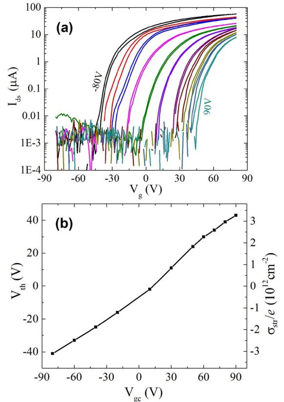
FIG. 6. (a) Effect of cooling the device from 350 K to 80 K under different applied gate voltages  $V_{gc}$  from  $-80$  V to  $90$  V. All the curves measured at 80 K and for  $V_{ds} = 1$  V show negligible hysteresis. (b) Variation of  $V_{th}$  with  $V_{gc}$ . The axis labels on the right in (b) show the corresponding blocked slow trap density.
