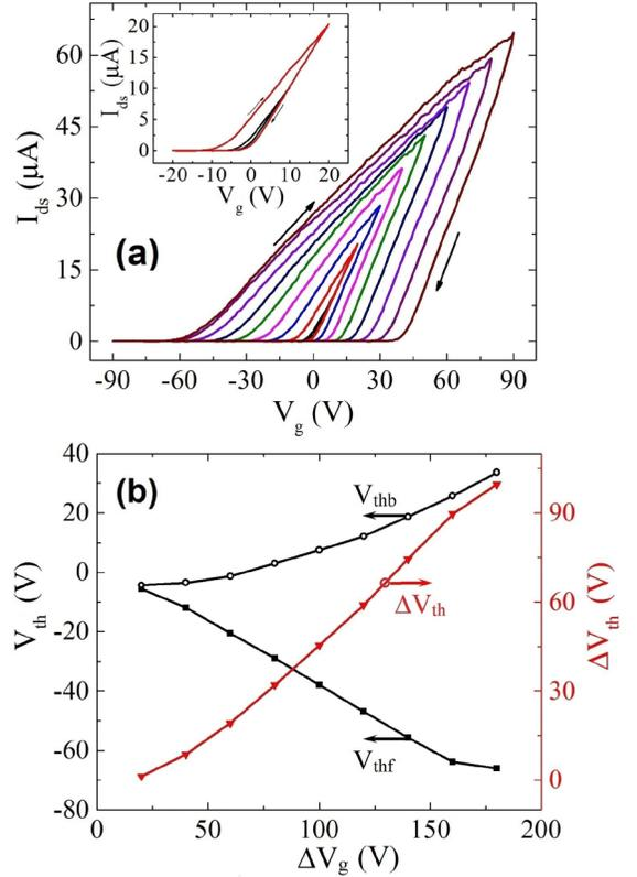
FIG. 3. (a)  $I_{ds}$  versus  $V_g$  at  $V_{ds} = 1$  V for different sweep ranges of  $V_g$  from  $\pm 10$  to  $\pm 90$  V. All these curves are acquired at the same  $V_g$  sweep rate. The inset shows the zoomed-in portion for  $\pm 10$  and  $\pm 20$  V range  $V_g$  sweeps. (b) Variation of  $V_{thf}$ ,  $V_{thb}$ , and  $\Delta V_{th}$  with sweep range  $\Delta V_g$  as extracted from (a).
