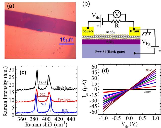
FIG. 1. (a) Optical image of few-layer MoS<sub>2</sub> with gold contacts. (b) The electrical schematic drawing of MoS<sub>2</sub> FET. (c) Raman spectra measured on exfoliated single layer, few-layer, and bulk MoS<sub>2</sub>. (d)  $I_{ds}$  versus  $V_{ds}$  for a few-layer device at different gate voltage values.
