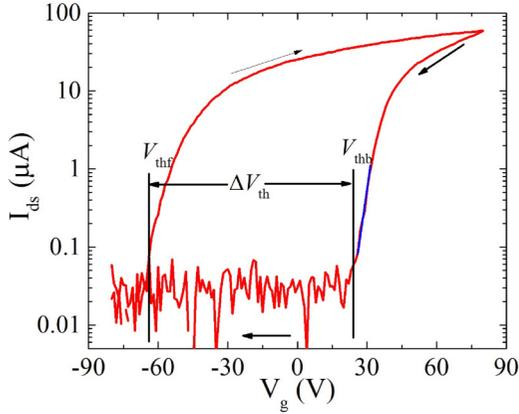
FIG. 2. The measured gate-dependent drain current for a few-layer MoS<sub>2</sub> at  $V_{ds} = 1$  V as a function of  $V_g$  and over a  $V_g$  cycle from 0 to  $-80$  V, then to  $+80$  and back to zero.
