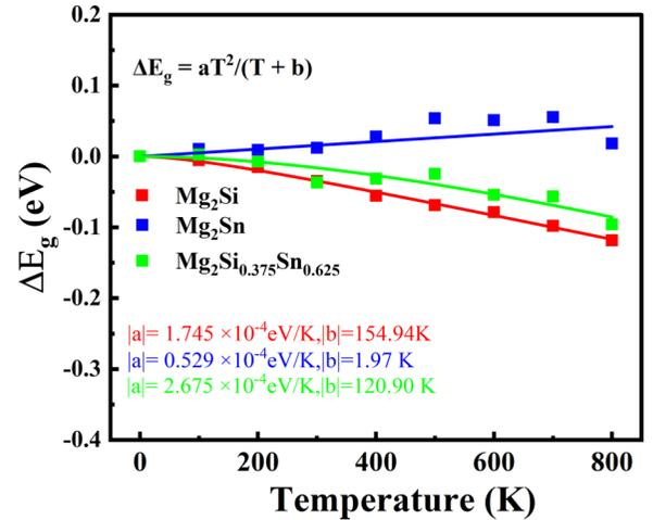
FIG. 5. The temperature-dependence gap of  $Mg_2Si$  (red),  $Mg_2Sn$  (blue),  $Mg_2Si_{0.375}Sn_{0.625}$  (green) with the corresponding nonlinear fittings by the Varshni equation of  $\Delta E_g = aT^2/(T + b)$ . The absolute values of coefficients  $|a|$  and  $|b|$  are listed, and the band gaps at 0 K are set as the references.
