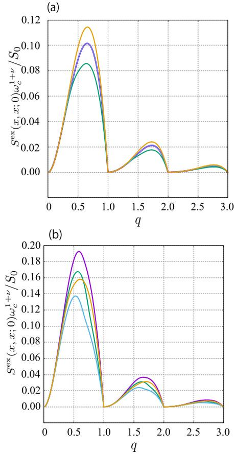
FIG. 4. Geometry dependence of the excess noise for (a) the two-lead case and (b) the one-lead case. We set the parameters as  $(L_1, \Omega) = (L/3, 3\pi v_N/2L)$  (purple line),  $(L/2, 2\pi v_N/L)$  (green line),  $(2L/3, 3\pi v_N/2L)$  (blue line), and  $(L/2, \pi v_N/L)$  (orange line). The other parameters are set as  $\eta = 0.1$ ,  $\omega_c/\Omega = 100$ , and  $g_N = 0.2$ .
