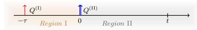
FIG. 1. Pulsed excitation scheme showing a sequence of ultra-short laser pulses with a positive delay time \tau . The first pulse with the pulse area \mu_{c_1}\mathcal{E}_I and action Q^{(I)} on the DM arrives at t_1 = -\tau . After delay \tau , two identical pulses with the resulting pulse area \mu_{c_{II}}\mathcal{E}_{II} and the total action Q^{(II)} arrive together at t_{II} = 0 . The observation time is denoted by t .
