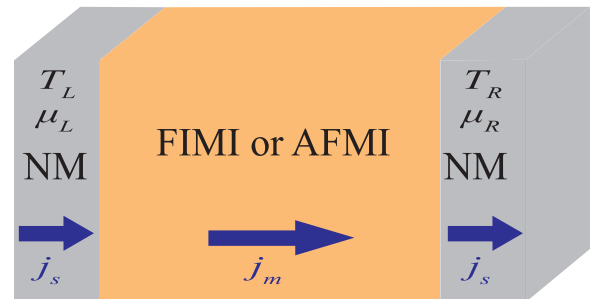
FIG. 2. Schematic diagram that illustrates the transport of magnon current through FIMI or AFMI driven by temperature or spin chemical potential step.
