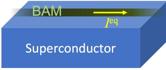
FIG. 1. Depositing a BAM wire on a conventional SC will generate an equilibrium current I^{\text{eq}} , a SDE in general, and a perfect SDE with unit diode coefficient if the band asymmetry exceeds a threshold determined by the critical Cooper pair momentum of the parent SC. (See text for details.)
