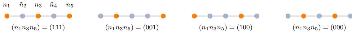
FIG. 11. The line graph is the only connected blockade graph on five vertices with (at least) four maximal independent sets (orange vertices), (at least) one of which has (at least) three vertices. To realize the state (111), the vertices \{1, 3, 5\} must be chosen as ports, with 3 as output; the four maximal independent sets then realize the truth table of AND (these four states cannot be made degenerate while maintaining a gap, see text).
