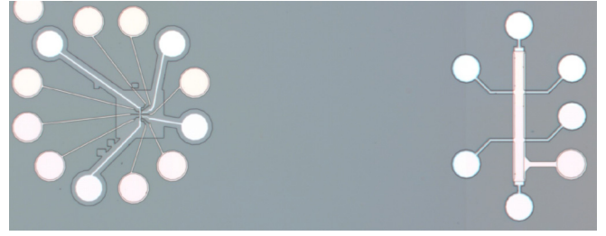
FIG. 5. There are Hall bars on the same chip as our topological gap devices, visible at the right and left sides, respectively, of this optical image. Both device types undergo the same processing steps, so the charged defect density at the semiconductor-dielectric interface n_{2\text{D,int}} extracted from Hall mobility measurements is reflective of the semiconductor-dielectric interface in the neighboring topological gap device.
