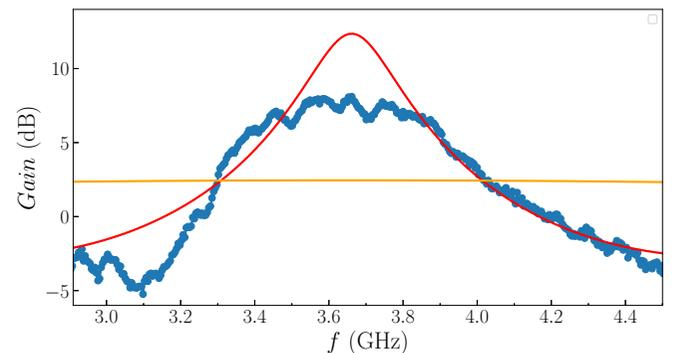
FIG. 6. The measured gain of the TWPA (blue line) for the pump frequency of 3.38 GHz. Orange and red curves are the results of the standard CME and the model with reflections for  $\Gamma_p = 0.72$ , respectively.
