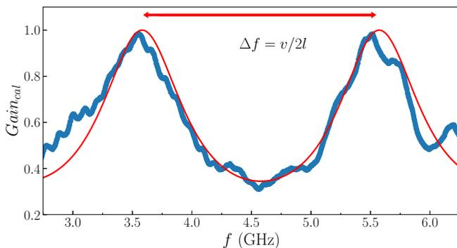
FIG. 5. (a) Calibrated weak signal transmission without pumping tone (blue line). Fit of the data by Fabry-Pérot oscillating transmission (9) (red curve). The parameters of the fit,  $\Gamma_s$  and  $v$ , are listed in Table II.
