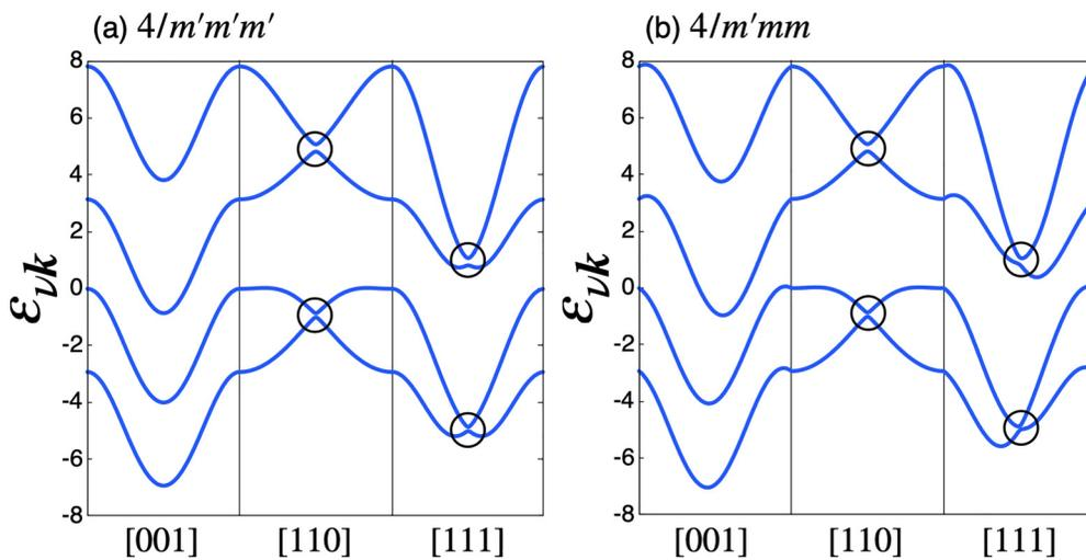
FIG. 3. Band structures for the magnetic orderings with (a)  $M_u$  under the magnetic point group (MPG)  $4/m'm'm'$  and (b)  $T_z$  under the MPG  $4/m'mm$ . In each panel, the wave number  $(k_x, k_y, k_z)$  dependence is as follows:  $(k_x, k_y, k_z) = (0, 0, 2s)$  in [001],  $(s, s, 0)$  in [110], and  $(s, s, 2s)$  in [111] with  $0 \leq s \leq \pi$ . The circles indicate the narrow band gap region.
