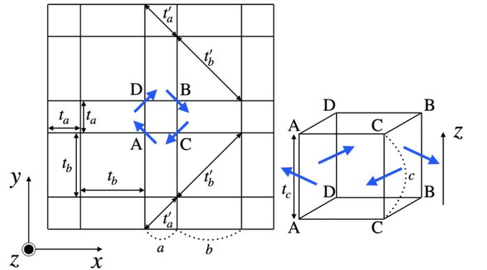
FIG. 1. The four-sublattice layered tetragonal structure with the hopping parameters ( $t_a, t_b, t'_a, t'_b, t_c$ ) and  $g$  vector denoted as the blue arrows in our model in Eq. (13).  $a, b$ , and  $c$  are the lattice constants.
