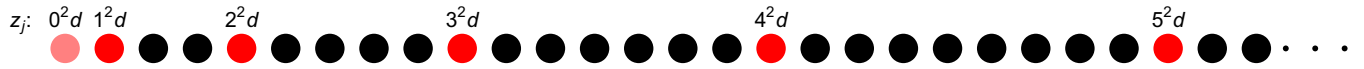
FIG. 1. Schematic diagram of the quadratic chain. z_j = j^2 d labels positions of lattice sites (or atoms) (pink for j = 0 , red for j \in \mathbb{N} ) comprising the quadratic chain. The scattering amplitude of the sites in black is zero. The Fourier transform of this chain is the Jacobi theta function \vartheta_3(q) with q the nome leading to a highly complex structure factor despite the quadratic chain's simplicity.
