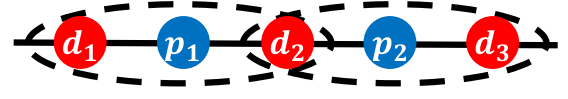
FIG. 9. An illustration of the one-dimensional d - p chain, where red atoms represent d sites while blue atoms represent p sites, and each atom is labeled by white letters. The black dashed ellipses are the clusters used in the cluster slave-bond calculation.
