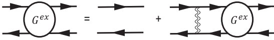
FIG. 3. The Feynman diagram of the screened-ladder approximation for G^{ex} . The upper and lower solid lines with rightward and leftward arrows are electron propagators in the b band and a band, respectively. The double wavy line is the screened Coulomb interaction w(\mathbf{y}) or w(\mathbf{k} - \mathbf{k}') represented by the Feynman diagram in Fig. 4.
