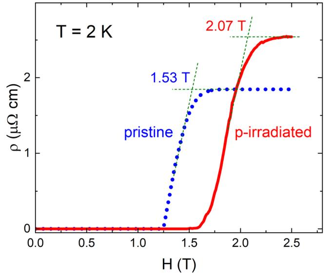
FIG. 4. Resistivity at  $T = 2$  K as a function of a magnetic field before (dotted blue line) and after (solid red line) the proton irradiation. The upper critical field increases from 1.53 T before irradiation to 2.07 T after.
