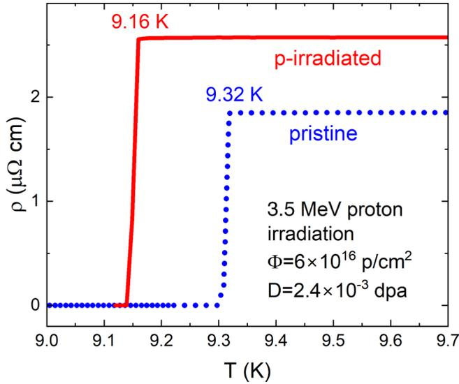
FIG. 3. Resistivity of 160 nm niobium film on a silicon substrate in the vicinity of the superconducting transition,  $T_c$ . The blue dotted line shows the pristine state, and the solid red line is the same film after proton irradiation. The superconducting transition temperature shifts by,  $\Delta T_c = 9.32 - 9.16 = 0.17$  K, while the resistivity just above the transition changed by  $\Delta\rho(T_c) = 2.59 - 1.87 = 0.72 \mu\Omega \text{ cm}$ .
