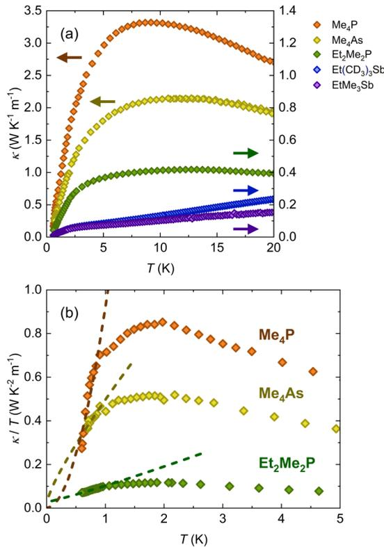
FIG. 2. (a) Temperature dependence of the thermal conductivity  $\kappa$  of the  $\beta'$ -X[Pd(dmit)<sub>2</sub>]<sub>2</sub> series shown as a  $\kappa$  vs  $T$  plot. (b)  $\kappa/T$  vs  $T$  plot of the antiferromagnetic salts below 5 K. The dashed lines denote the free power-law fitting curve  $\kappa/T = a + bT^c$  for the data below 1 K. The fitting parameter is shown in Table S1.
