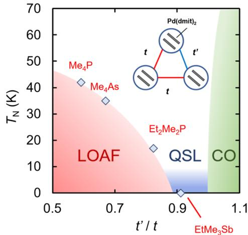
FIG. 1. Phase diagram of electronic and magnetic states of the  $\beta'$ - $X[\text{Pd}(\text{dmit})_2]_2$  series as a function of the frustration parameter  $t'/t$ . The QSL state appears between the long-range antiferromagnetic order (LOAF) phase and the nonmagnetic charge order (CO) phase.
