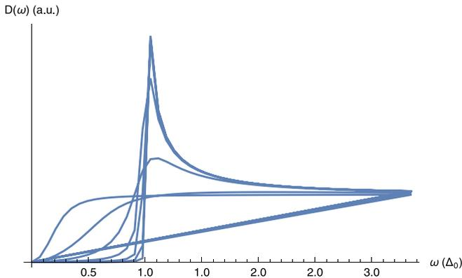
FIG. 6. Relation between the density of states and the electron energy when  $\Delta$  is set to be different values. The case with von Hove singularity corresponds to the situation in low temperatures.
