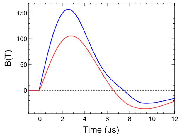
FIG. 2. Waveforms of the pulsed magnetic fields generated by means of the single-turn coil. The vertical-type (red curve) and horizontal-type (blue curve) single-turn coil field generators were utilized for generations of fields of up to 105 and 160 T, respectively [8].
