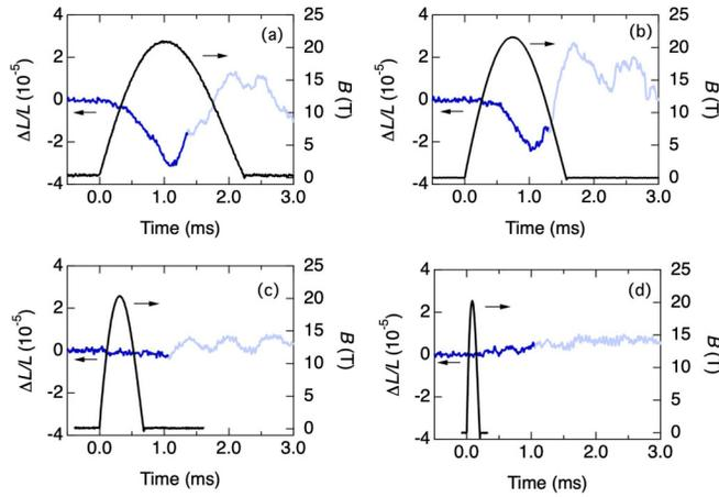
FIG. 8. The magnetostriction  $\Delta L/L$  and the magnetic field are plotted as a function of time.
