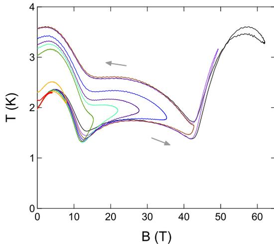
FIG. 6. Magnetocaloric effect at the initial temperature of 2 K with several maximum field strengths.
