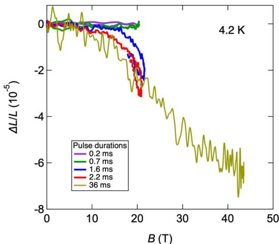
FIG. 9.  $\Delta L/L$  measured with a longer magnetic field pulse of up to 42 T is plotted as a function of magnetic field along with the results shown in Figs. 8(a) to 8(d).
