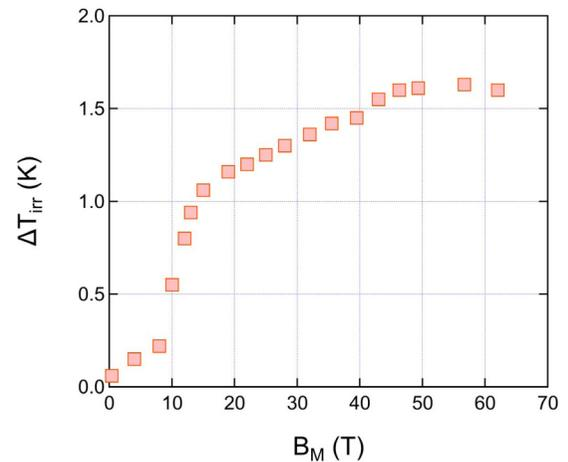
FIG. 7. Temperature difference  $\Delta T_{\text{irr}}$  between the initial and final temperatures measured in the MCE experiment.  $\Delta T_{\text{irr}}$  depends on a maximum value of a pulsed magnetic field  $B_M$ .
