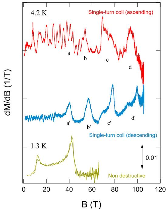
FIG. 3.  $dM/dB$  curves in the field-ascending (red) and field-descending (blue) processes are shown for the single-turn coil experiment up to 105 T.  $dM/dB$  curve in the nondestructive 5-ms-pulsed magnetic field is shown with dark yellow line.
