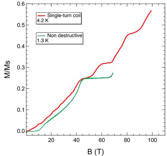
FIG. 1. Magnetization process of a single crystal of BIP-TENO measured with the  $\mu\text{s}$  single-turn coil (red curve). The green curve shows the magnetization process of BIP-TENO measured in a non-destructive pulsed magnetic field with a duration of 5 ms [7].
