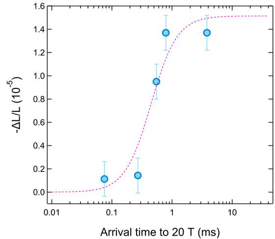
FIG. 10.  $-\Delta L/L$  at 20 T is plotted as a function of a time required to reach 20 T. The dashed curve is a guide for eyes.
